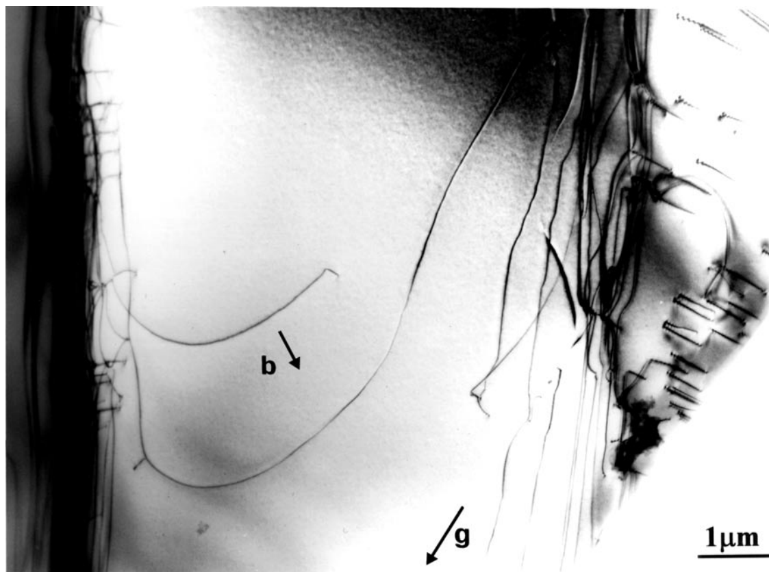
Figure 2. A plan-view sample of ELOG GaN which has been tilted to show threading dislocations in the seed crystal (right-hand side) obliquely inclined, the boundary between the seed crystal and the laterally overgrown material (right) and the boundary between laterally overgrown crystals (left). The image is taken under two-beam diffracting conditions with g = \langle 11\bar{2}0 \rangle . The two a -type dislocations in the mainly defect free central region (Burgers vector shown) are believed to have propagated under shear stresses generated during cooling immediately after film growth. (Courtesy of Z Liliental-Weber).
